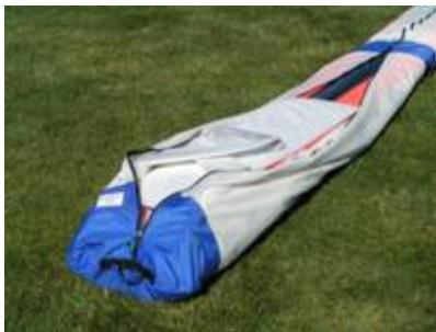
2. Remove the basetube from the D-Cell and raise the uprights. Do not allow the uprights to inadvertently fall. This could damage the sail, D-cell or the #1 rib. When installing the base tube, it's best to **stand**
