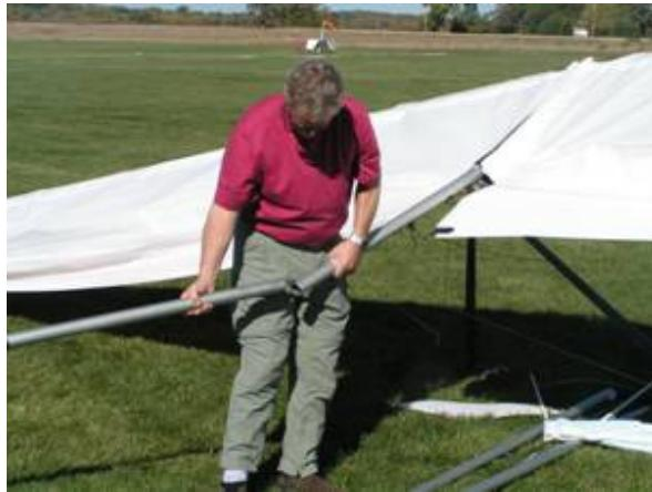
10. Collect the aluminum tube and carbon ribs and wing tip for one wing. The left wing components are marked with red spots - the right with green. On the ribs, there's an indication on the colored spot, of the edge that goes up. Remove the wing tip bag - you can roll it and secure with the Velcro strap or stuff in your back pocket. The description from here is based on the left wing assembly and you will have to mirror that process for the right.
