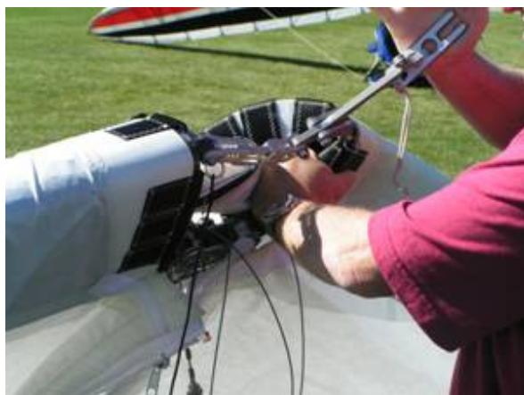
9. Walk to the rear of the keel, lift it and insert the stinger being sure hear both pins snap in place in the
