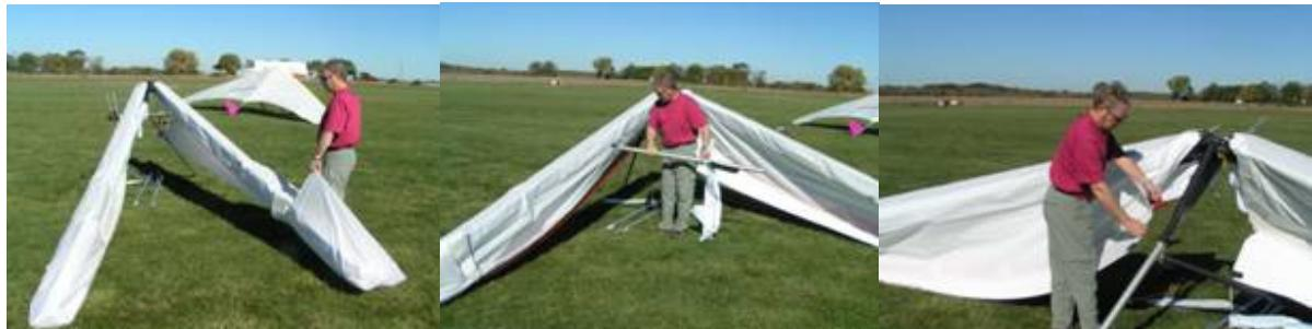
7. Connect the sail rings to the bracket at the top of the control frame by depressing the pin in the center of that bracket (picture below). Make sure you hear the pin snap shut locking the rings in place. **Note : Be very cautious of the flaps. Do NOT twist them or bend beyond a 20 degree angle.**
