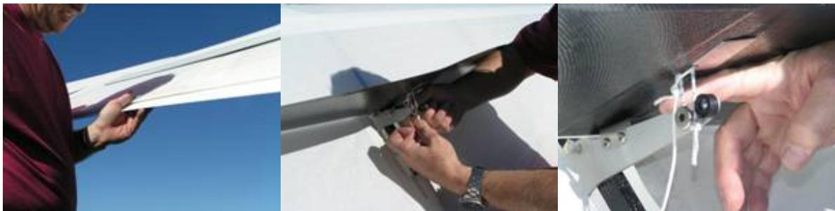
18. Next cam in place the rib with the spoiler arm mechanism. If you learn to control the fish cam with your left hand and the rib with your right (palms up - see the picture), you'll find that to be the quickest technique and require the least amount of the Velcro to be opened. It also saves your skin from the hook portion of the Velcro which is the most abrasive. After that, connect the bungee to the spoiler arm - this must also become part of your **Preflight Check**.
