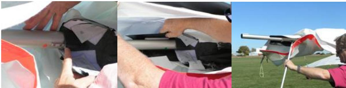
12. Slide the tube in aligning the key and the key slot until the tube bottoms out (pictured above). The carbon leading edge shell packs along the front edge. You'll be able to find it just outside the end of the D-cell as shown, slide it out along the aluminum extension tube. Now pull the sail outward so that you can bring the last fish cam around the tube end leaving the tube extending from the end of the sail (shown below).
