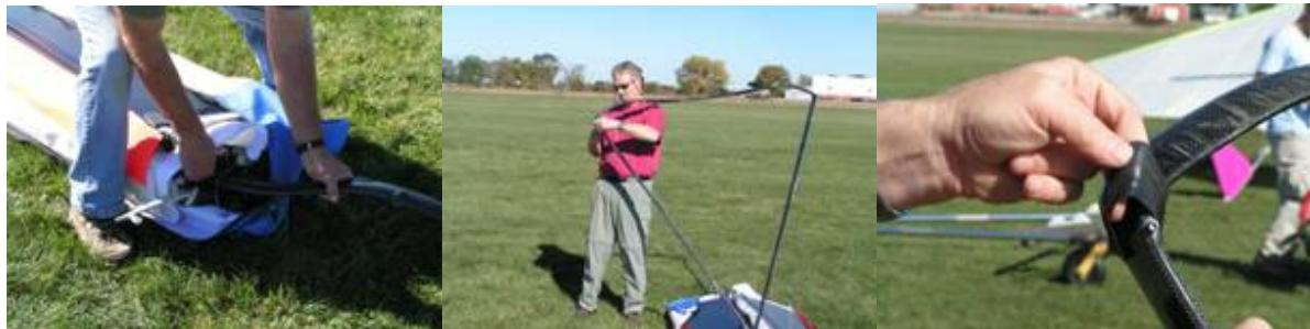
3. Stand the ATOS VR up on the control frame. **Important with uneven area:** The wing must stand stably on the control frame. If it should tilt against the top of the upright connection, the D-cell can be damaged or the sail compressed. It's easiest to lift the D-cells straight up with one hand while rotating the control frame underneath with the other.
