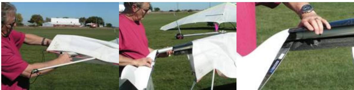
13. Depress the two pins on the Wingtip tube and slide it into the extension tube until they pop and the wingtip is solidly engaged. Slide the carbon leading edge extension out until it overlays the white wingtip.
