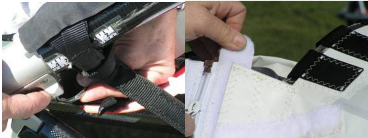
8. Engage the nose mechanism and with the cam tool, push the connection closed and insert the pip pin to secure it in place. The hook end of the latch must be **through and behind** the opposing piece to insert the pip pin. **Note - place your hands as shown and be cautious in this process that you do not allow your face to be close to and in front of the latch. If your hand or the tool were to slip off the latch, it would spring open forcefully and be potentially, very damaging.**
