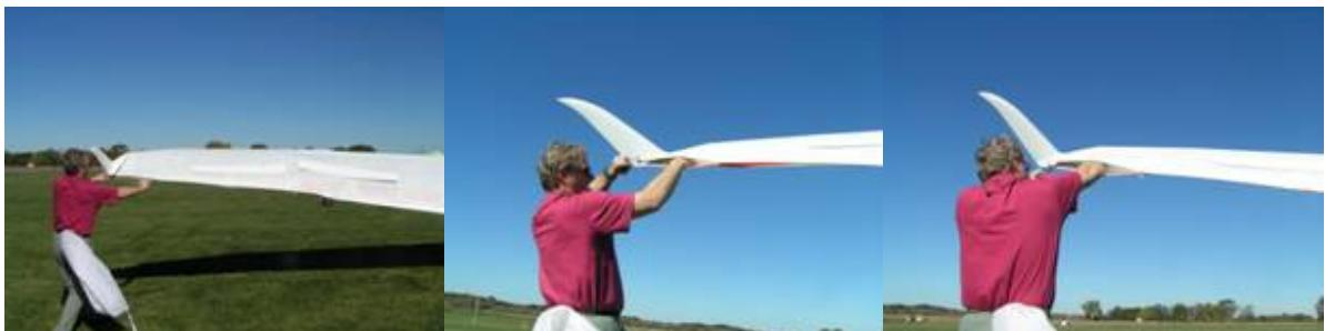
15. Now you want to rotate the tip lever around the tip wand end. Grasp the **upper lever end rope** in your left hand and the **lower lever end rope** in your right. The best action is to pull the left hand to the rear and guide the right hand into the sail and against the wand. Notice the left hand is below the wing tip and that both hands **remain in the same plane as the sail**. Please review the section on adjustments prior to your first setup.
