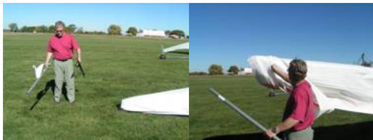
11. Start the tube end with the key into the last section of the sail (between the last and next to last fish cams) and rest the outer end on the ground. Stand behind the sail and open the Velcro of the third section to see the end of the D-cell. This will allow you to elevate the tube with your left hand as you guide it into the D-cell with your right making sure to not trap parts of the internal material.
