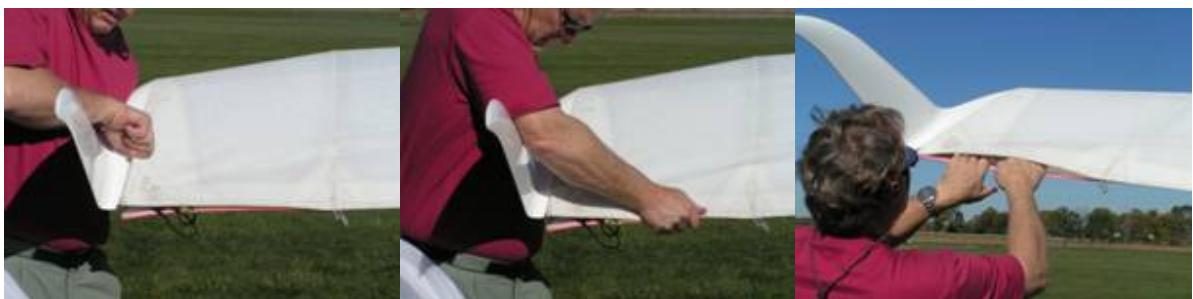
16. With your body against the wing tip, pull the sail edges out and toward the wingtip to allow you to properly fit and seal down the Velcro on the sail to the wing tip Velcro. Stuff the lever ropes into the sail and smooth out the sail. **Make sure you do not push on the upper part of the wing tip in this process.**
