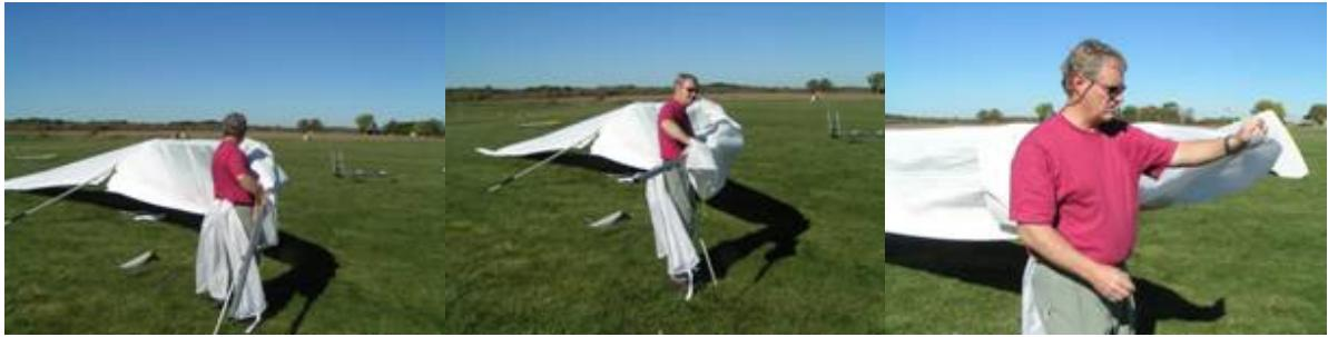
6. Remove the tip and then slide the extension tube out. Place the ribs, tip, and extension at the front of the glider so that they are not accidentally stepped on.
