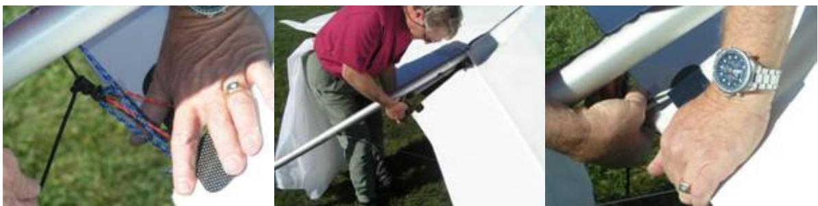
21. Pull the flap pins down and away from the keel in order to get enough room to insert the flap pins into the tabs on the flaps themselves. The above pictures show the sequence.
