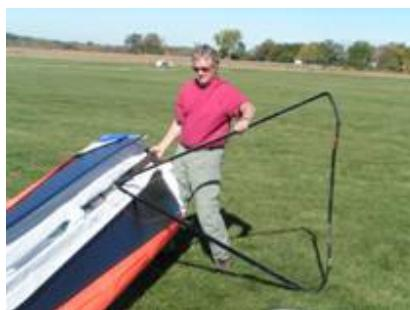
4. Remove all the parts from the D-Cell including the rib cam tool and the pull out the barrel ends of the spoiler wires. Stuff half the glider bag in the left and the rest in the right D-Cell.
