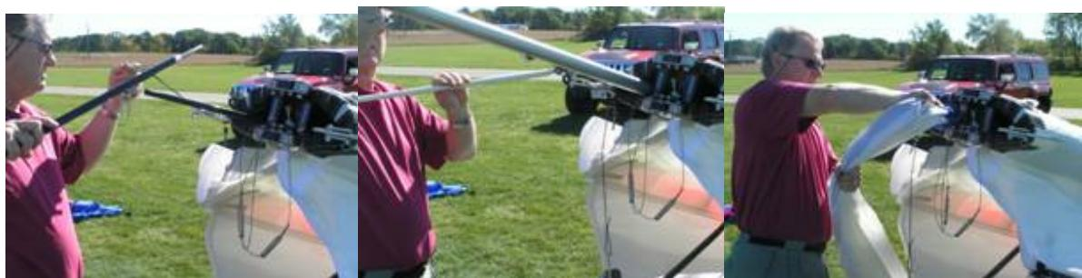
5. Prior to opening the wings, be sure that the two halves of the nose connection are opened wide out. If not, they could be compressed into the D-Cells or other parts by the nut-cracker action of opening the wings.
