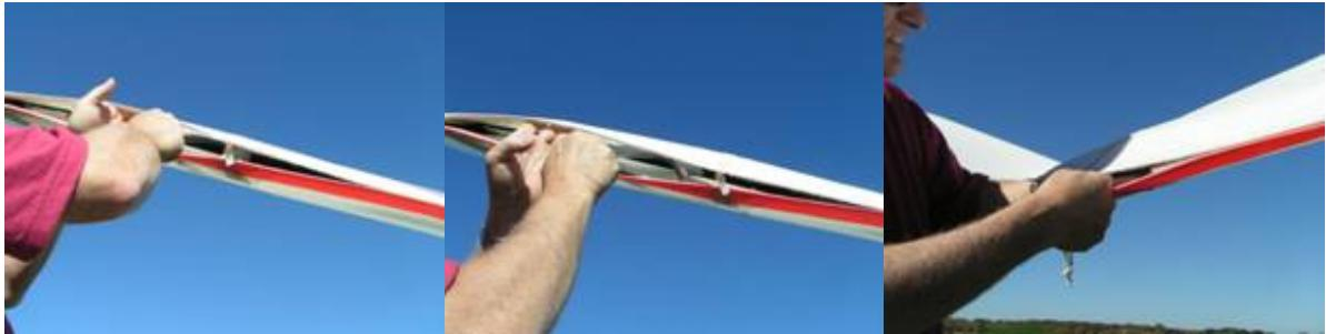
19. Now insert and cam in place the larger of the 2 outboard ribs and then the smaller. If you look in the sail, you can see the aluminum stop that they go against. Keep the sail aligned at the rear.
